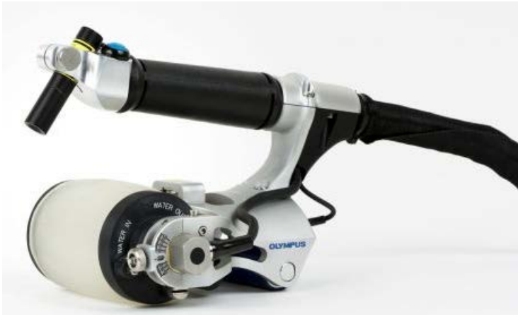
Figure 3: Image of 3.5MHz RollerFORM probe by Olympus used to scan TidGen® foils.
